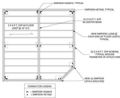
FLOOR FRAMING PLAN SCALE: 1/4" = 1'-0"
